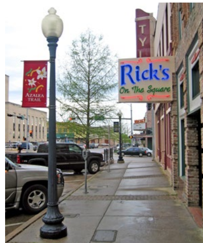
Acorn lights around the square are the right height for pedestrians but rather widely spaced for optimum light distribution.
