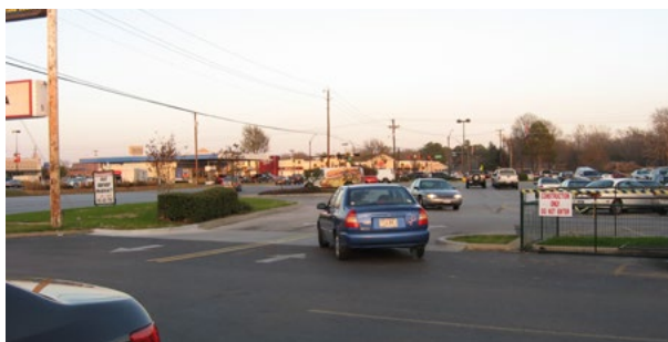
Adjacent shopping centers often do not have cross access (top), which forces drivers to return to the main road to reach the next driveway. Openings between shopping centers facilitate internal circulation and reduce traffic congestion on main highways (below).
